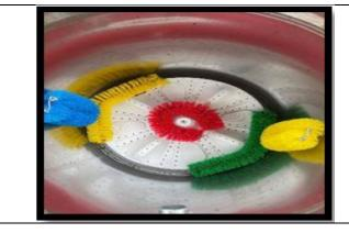
The inner core of design C is a combination of design A and design B. This design, however, has been very effective because it contains the best contact surface on the wall and below and flattens during the peeling process of onion skin.
