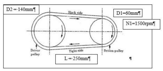
Figure 2: Belting system use in the project
