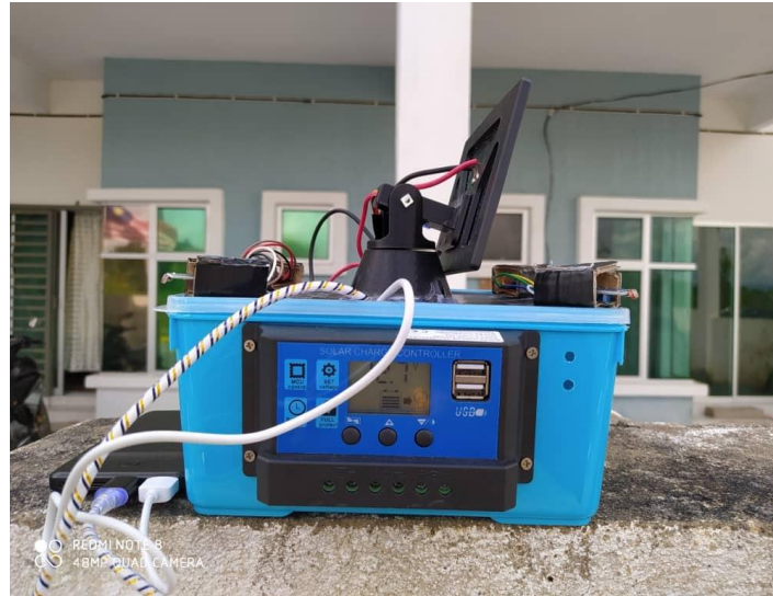
Figure 7: Dual-axis solar tracker on first day testing
