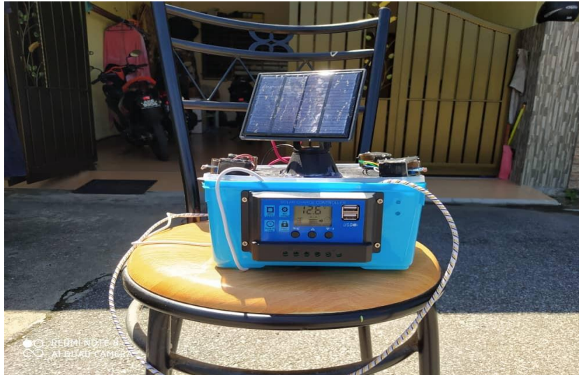
Figure 9: Dual-axis solar tracker position on second day testing
