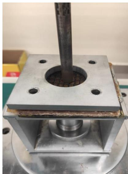
**Figure 7: Top view of the sample in compression testing**
