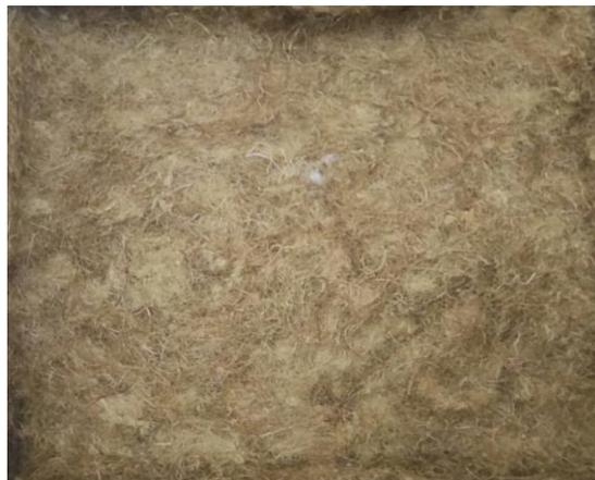
**Figure 4: Physical of bamboo fiber after undergoes opening process**
