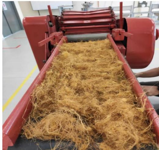
**Figure 3: Bamboo fiber undergoes opening process**
