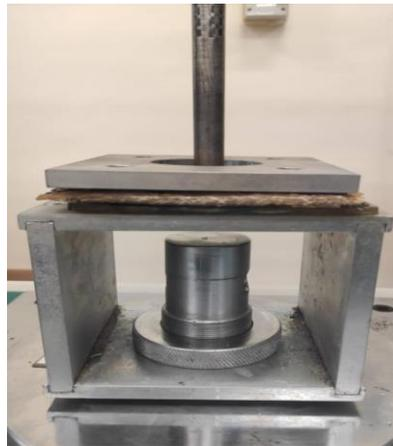
**Figure 6: Front view of sample in compression testing**
