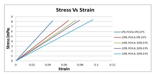
Figure 9: The graph of Stress vs Strain for concrete beam model
