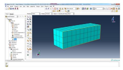
Figure 3: Mesh the concrete beam model
