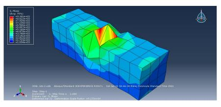
Figure 6: The deformation pattern for normal concrete beam
