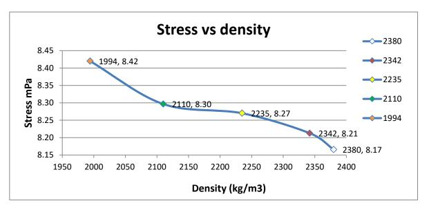
Figure 10: The graph of Stress against Density for concrete beam model
