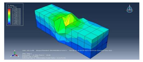
Figure 7: The deformation pattern for concrete beam containing 20.00 % POFA and 0.00 % EPS
