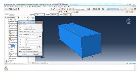
Figure 4: Point a Load and Boundary Conditions to model
