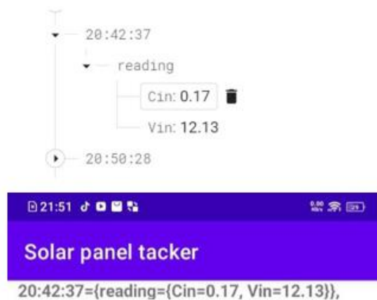
Figure 11: Real Time Monitoring from Load (Lamp)
