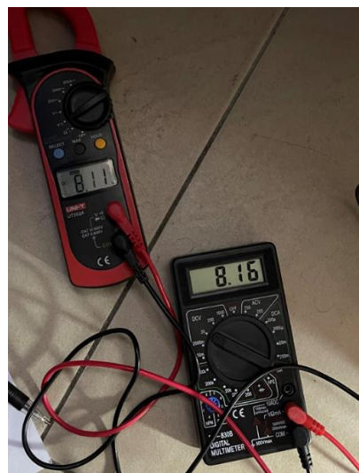
Figure 24: Measurements That Validate by Using Multimeters
