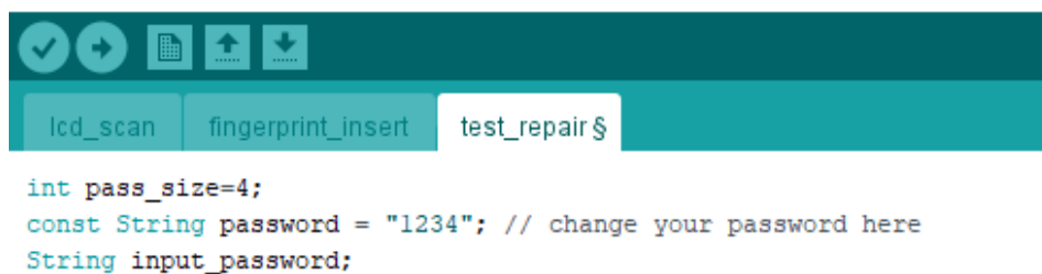
Figure 8: Set password for password code and fingerprint-based security using relay
