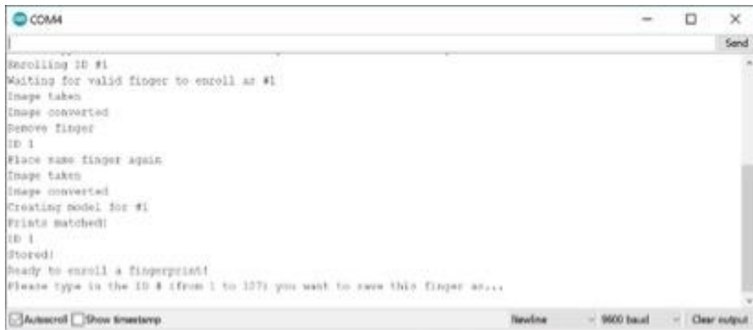
Figure 7: Image of fingerprint successfully stored in Arduino Un
