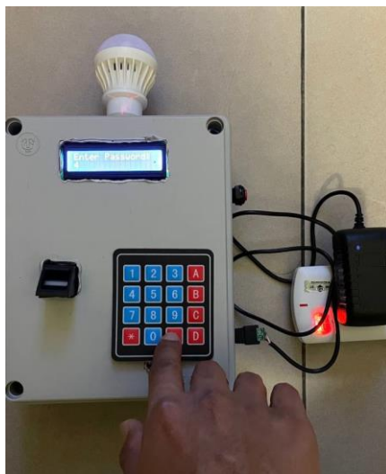
Figure 12: Fingerprint and password is matched; it triggers the relay and light up the bulb
