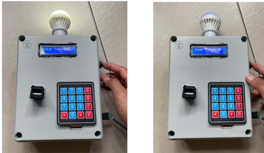
Figure 13: Emergency push button is triggered to cut off the load
