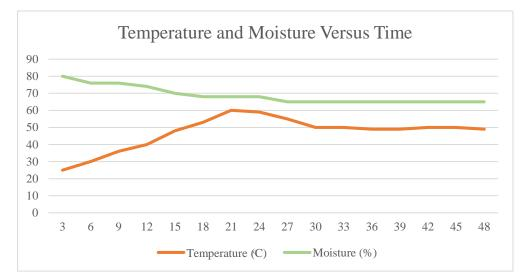
Figure 5: Graph of Temperature and Moisture versus Time for 48 hours
