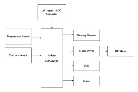
Figure 2: Fertilization of Food Waste Management block diagram
