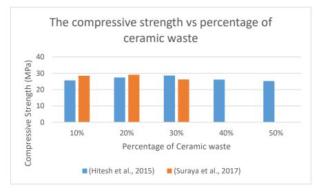
Figure 4: Bar chart of compressive strength at age 7 days
