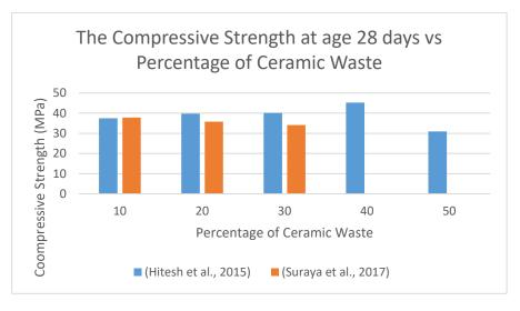
Figure 5: Bar Chart of compressive Strength at 28 days
