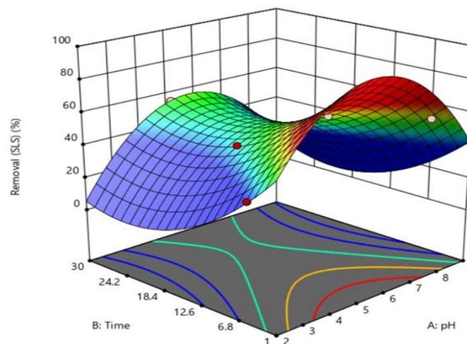
**Figure 4: Effects of pH and time on the removal of SLS**
