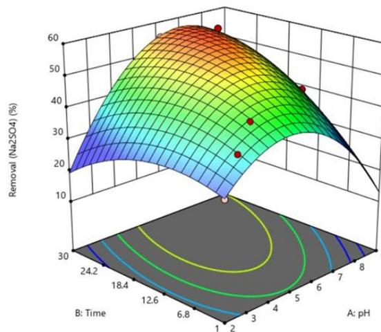
**Figure 3: Effects of pH and time on the removal of  $\text{Na}_2\text{SO}_4$**
