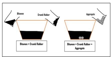
Figure 3: Wet method process
