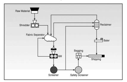
Figure 4: Crumb Rubber Process [4]
