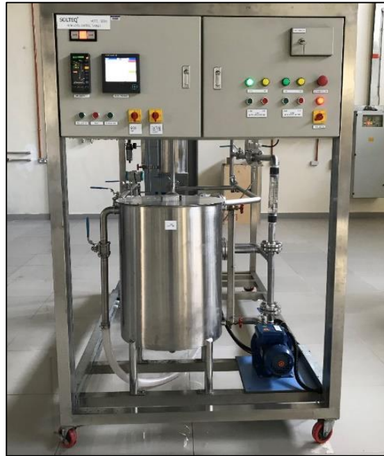
Figure 1: Level Flow Process Control Training System (Model SE 665)
