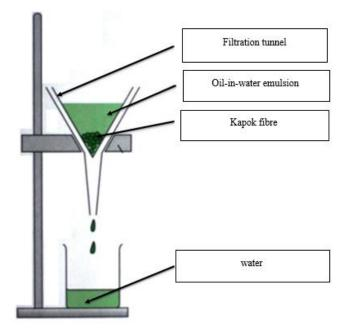
Figure 1: Apparatus of filtration system
