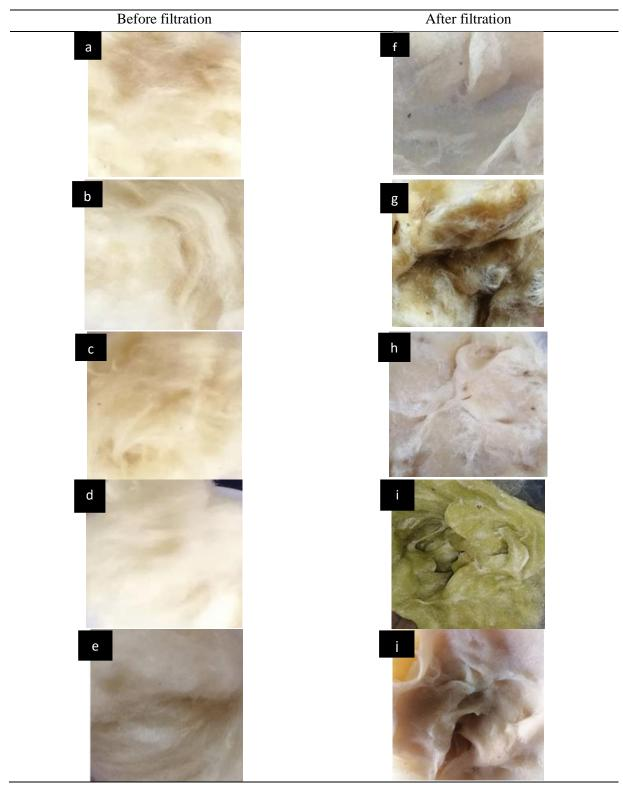
Table 3: Surface morphology of Kapok fibre before and after being treated with different oil
