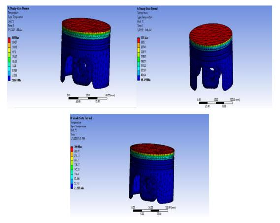
Figure 5: Temperature Distribution of Al Alloy, Gray Cast Iron and Si-C in Steady State Thermal Table 3: Minimum and Maximum Value of Temperature Distribution in Steady State
