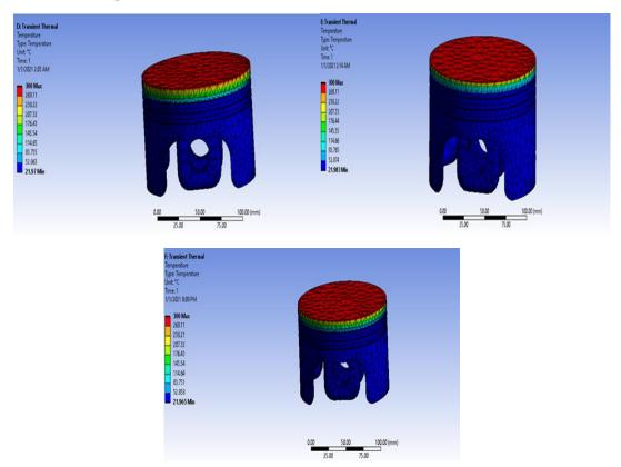
Figure 6: Temperature Distribution of Al Alloy, Gray Cast Iron and Si-C in Transient Thermal Table 4: Minimum and Maximum Value of Temperature Distribution in Transient
