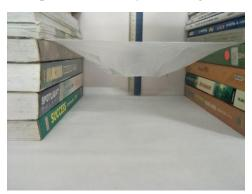
Figure 7: The plastic film was deformed after the 5.0 kg of load unloaded
