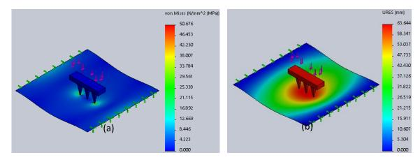
Figure 11: (a) The plastic film towards point stresses (b) displacement of the plastic film after acted by sample G
