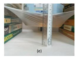
Figure 6: The loads with (a) 0.5 kg, (b) 1.0 kg, (c) 2.0 kg, (d) 5.0 kg (square base) and (e) 5.0 kg (cylinder base) acted on the plastic film
