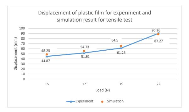
Figure 5: Displacement of plastic film for experiment and simulation results for the tensile test
