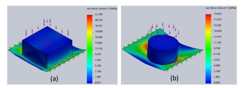
Figure 9: Stress on plastic film after acted on (a) 5.0 kg (square base) and (b) 5.0 kg of load (cylinder base)
