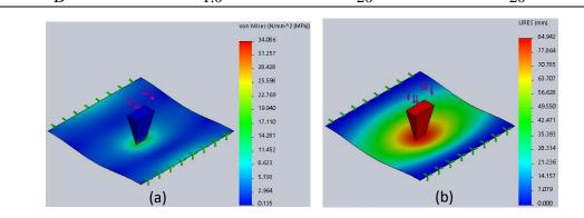
Figure 10: (a) The plastic film towards edge stresses (b) displacement of the plastic film after acted by sample D
