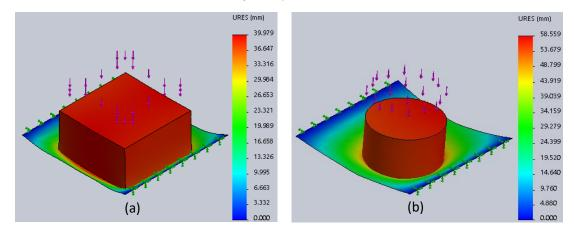
Figure 8: Displacement of plastic film with (a) 5.0 kg (square base) and (b) 5.0 kg of load (cylinder base)
