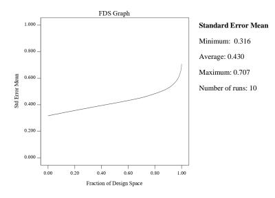
Figure 2: Fractional of design space for response surface design with minimum 10 number of runs
