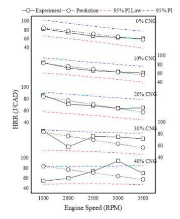
Figure 13: Predicted vs Experiment value for HRR model
