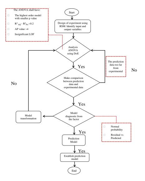
Figure 3: The process of flow chart for development prediction model
