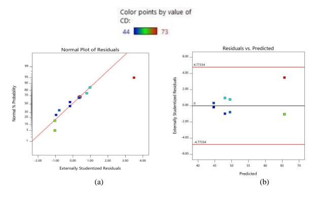
Figure 8: Diagnostic plot for Combustion Duration model (a) Normal Plot of Residuals (b) Residuals vs Predicted
