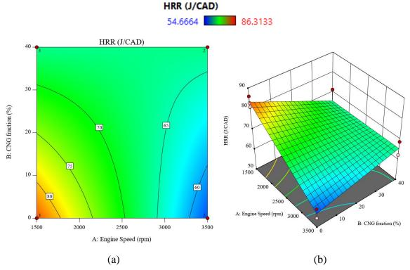
Figure 7: The contour plot (a) and response surface profile (b) for HRR model
