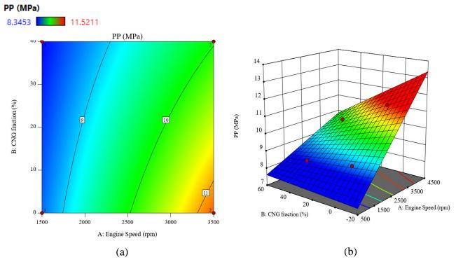
Figure 5: The contour plot (a) and response surface profile (b) for PP model
