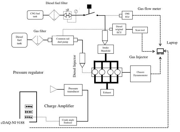
Figure 2: Schematic Diagram for experiment Setup
