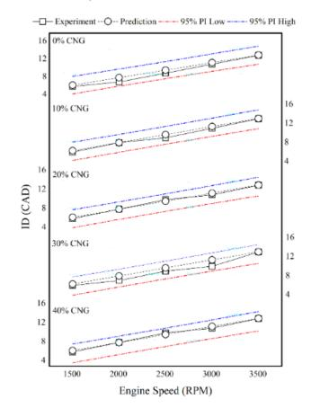
Figure 10: Predicted vs Experiment value for ID model
