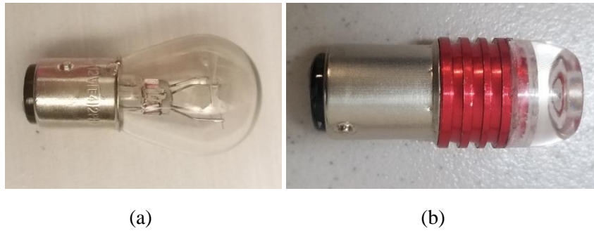
Figure 7: Bulbs used in the experiment; (a) Conventional, (b) Flashing
