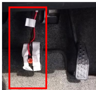
Figure 4: Push button attached to the brake pedal
