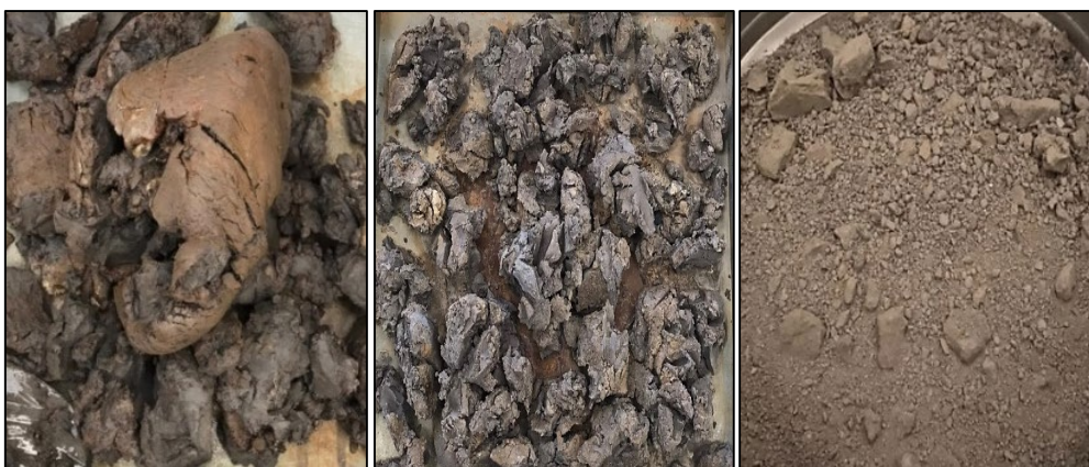
Figure 2: Soil sample dried (a) Original soil sample (b) Dried soil sample (c) Sample after grained
