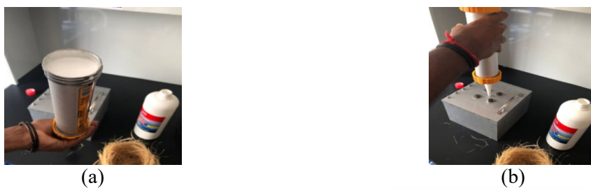
Figure 10: Glue test setup; (a) Glue filled up in the glue injector, (b) Glue injector place in the centre hole of the upper plate
