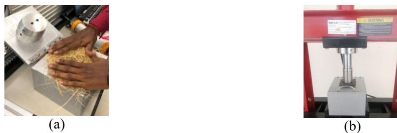
Figure 8: Compression test; (a) Bamboo fiber placed on mold cavity, (b) Compressed using compression machine
