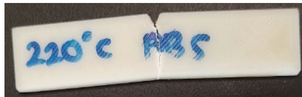
Figure 6: Izod impact test specimens after test
