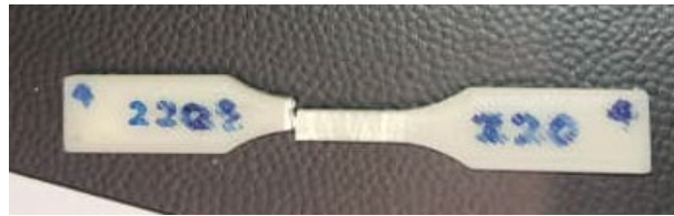
Figure 5: Tensile test specimens after test
