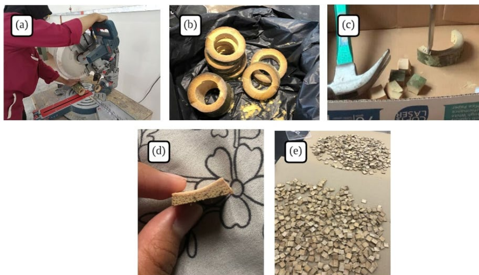
Figure 1: Raw material preparation: (a) process of cutting bamboo culm, (b) top section of bamboo, (c) chipping process of bamboo strips, (d) drying process in the open air
