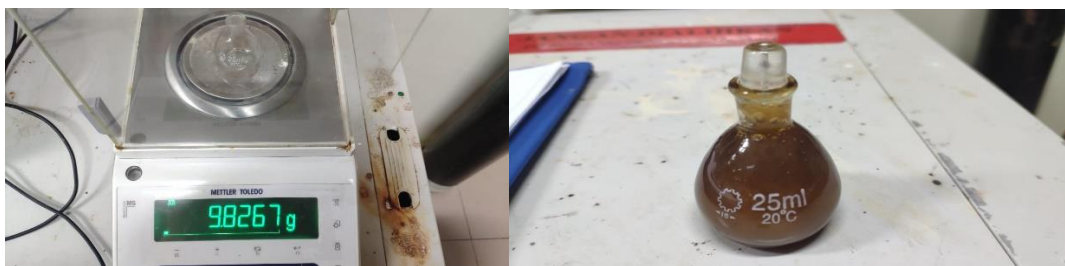
Figure 14: Mass of pycnometer and oil sample
