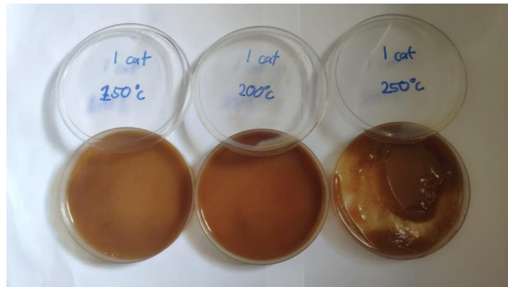
Figure 10: 1 nickel catalyst yield with different temperature
