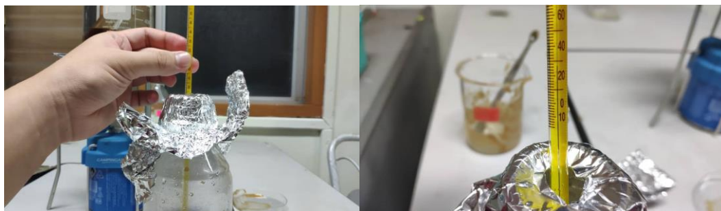
Figure 19: Latent heat test on pyrolysis oil
