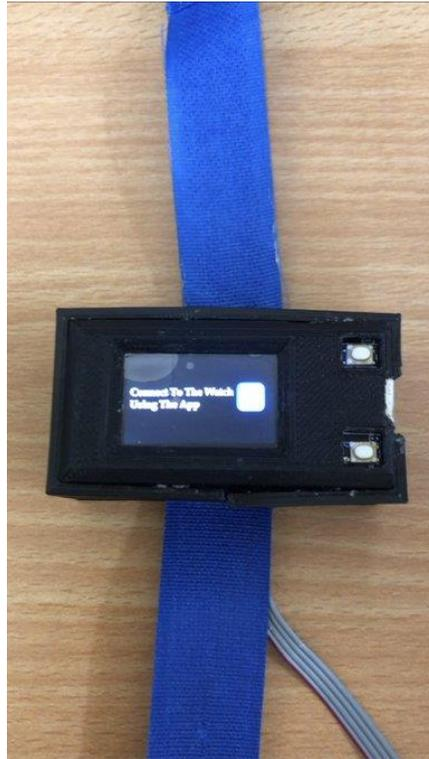
**Figure 5: Prototype of Smartwatch**
