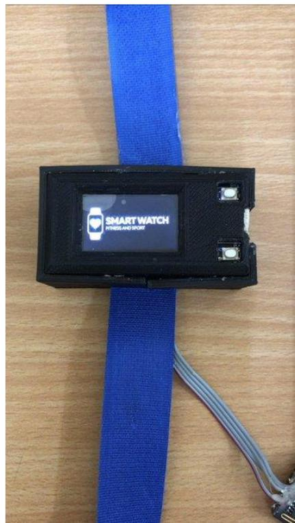
**Figure 4: Prototype of Smartwatch**
