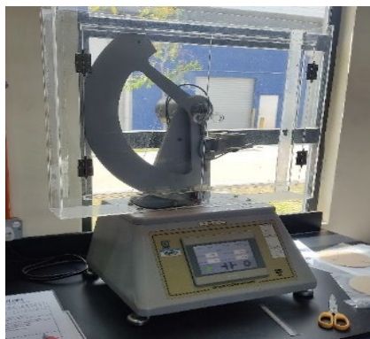
Figure 7: Equipment for tearing test
