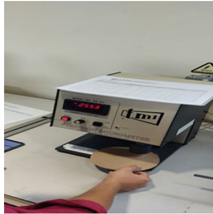
Figure 5: Thickness test process
