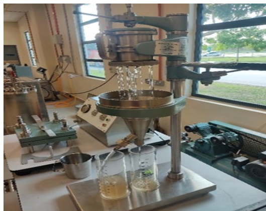
Figure 4: CSF Freeness test
