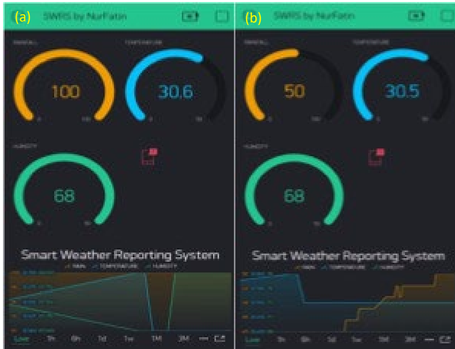
Figure 10 (a): Parameters readings during no rain; (b) Environmental readings when there is rain
