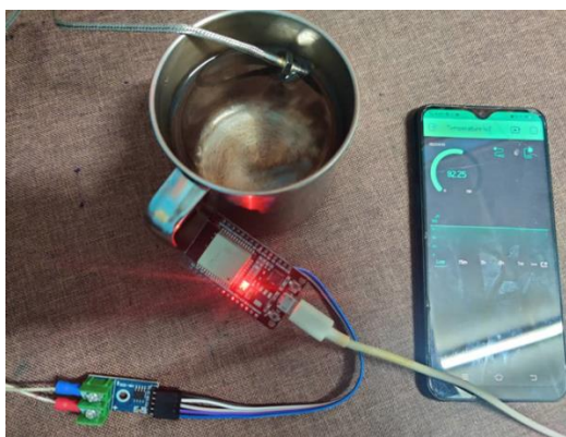
Figure 3: Temperature Sensor (MAX6675) Interfaced with NodeMCU (ESP32)
