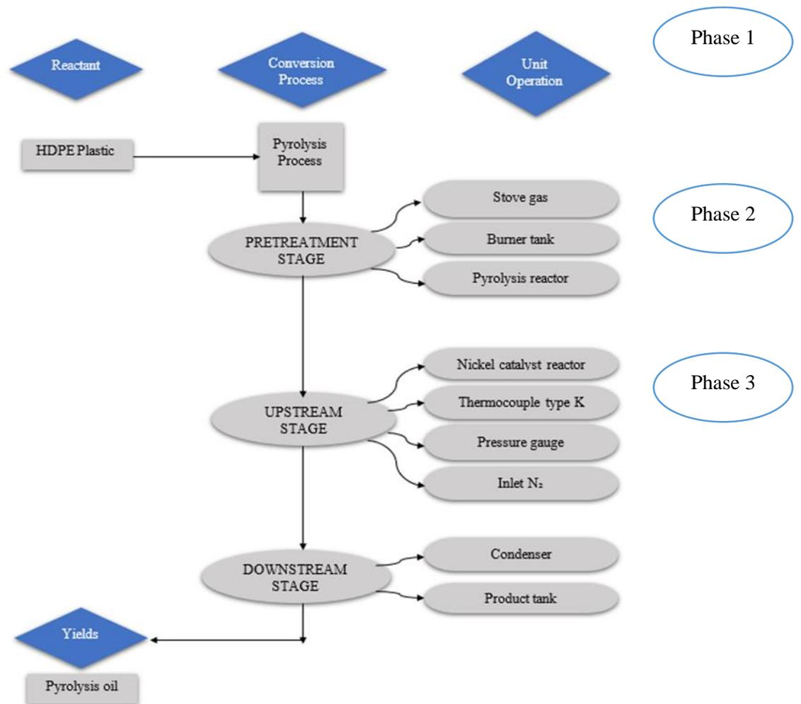
**Figure 1: Basic Flow Diagram (BFD) and Unit Operation Involves in Multistage Reactor Pyrolysis Process**
