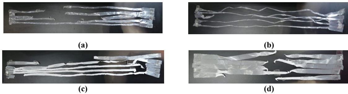
Figure 8: Specimen (a) A1, (b) A2, (c) B1 and (d) B2 undergo tensile test
