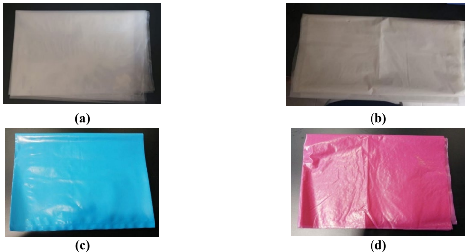
Figure 7: (a) Virgin LDPE from Wahdah, (b) Recycled LDPE from Wahdah, (c) Commercial virgin LDPE, (d) Commercial recycled LDPE
