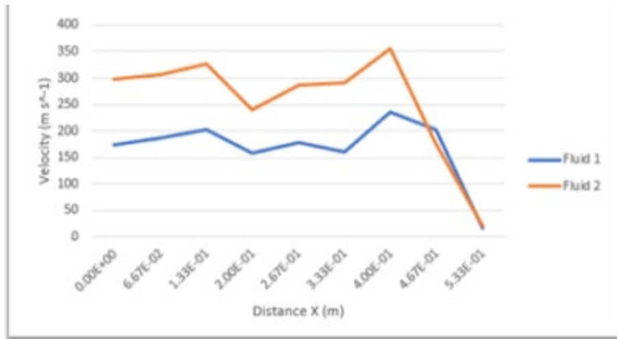
Figure 5: Velocity of fluid at centre of pipeline
