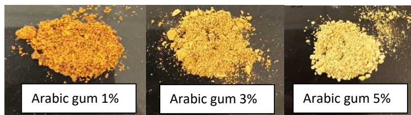
Figure 7: The colour of turmeric powder at 190 °C inlet temperature with different concentrations of arabic gum carrier
