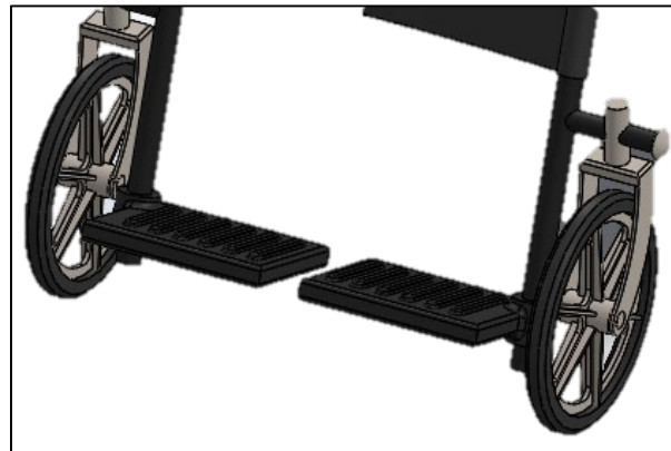
Figure 9: Adjustable leg rest design
