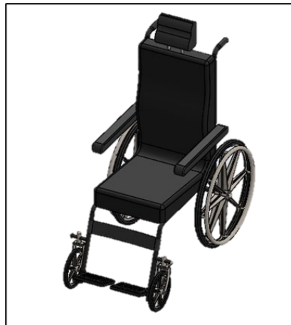
Figure 4: Proposed manual rigid frame wheelchair design
