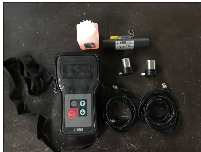
Figure 2: Ultrasonic Pulse Velocity (UPV) test
