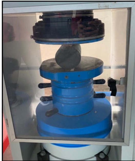
Figure 4: Splitting test on Concrete Cylinder
