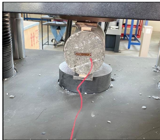
Figure 5: Split cylinder test with strain gauge
