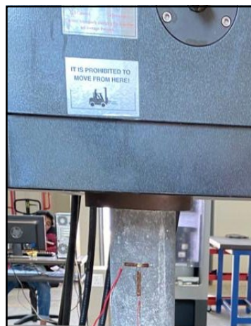
Figure 3: Strain gauge on Concrete Cylinder
