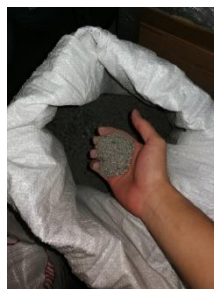
Figure 2: Palm oil boiler bottom ash
