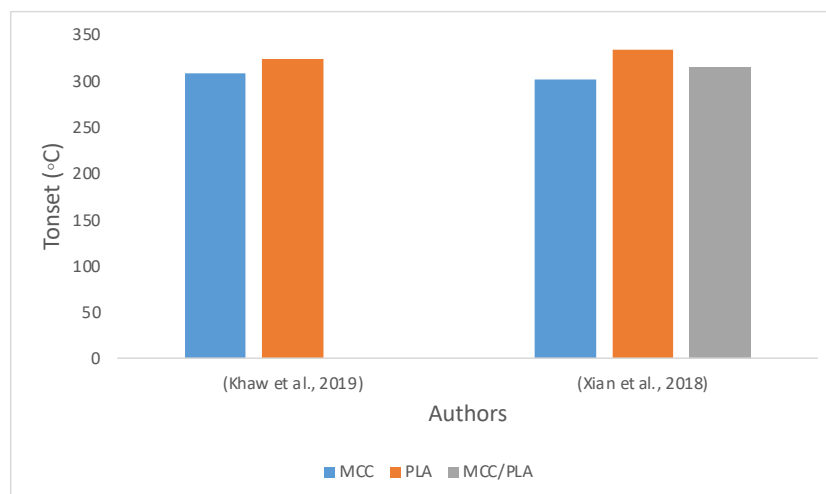
Figure 4: The comparison of CNC degradation onset before and after reinforcement with PLA composite
