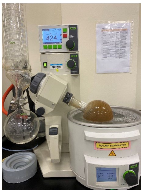
Figure 2: Ethanol recovery using rotary evaporator
