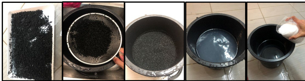
Figure 3: Process of crumb rubber treatment with sodium hydroxide solution
