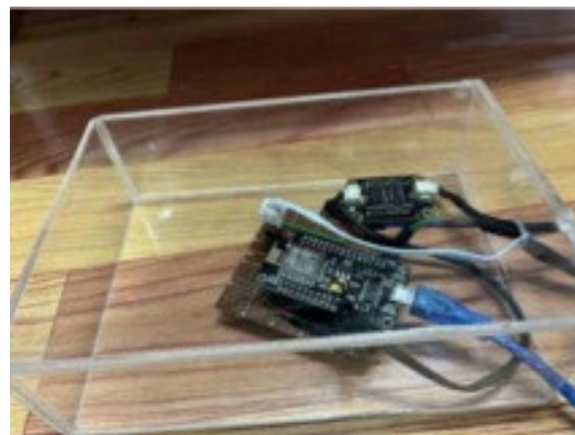
Figure 4: Acrylic casing for main control circuit (top view)
