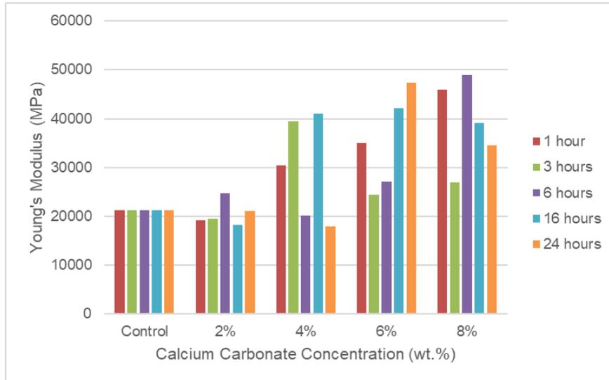
**Figure 3: Young's modulus of the bamboo fibre with various concentration and immersion duration**
