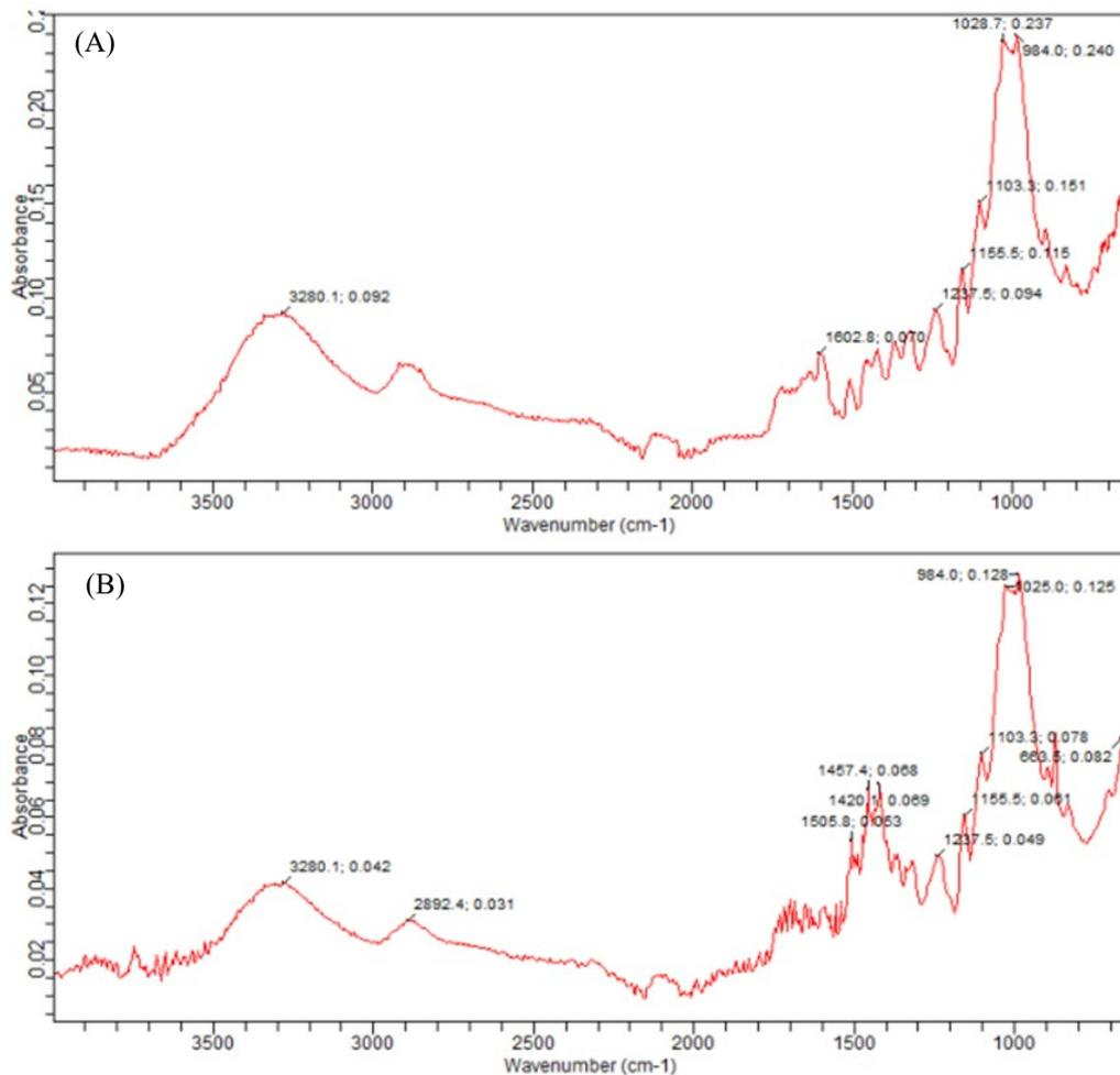
**Figure 6: The graph of FTIR analysis where (A) untreated bamboo fibre; (B) treated bamboo fibre**
