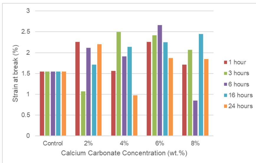
**Figure 4: Percentage of the strain-a-break of the bamboo fibre with various concentration and immersion duration**
