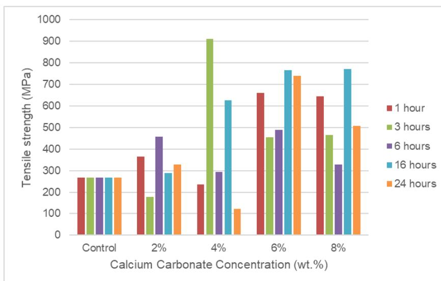
**Figure 2: The tensile strength of bamboo fibre with various concentration and immersion duration**
