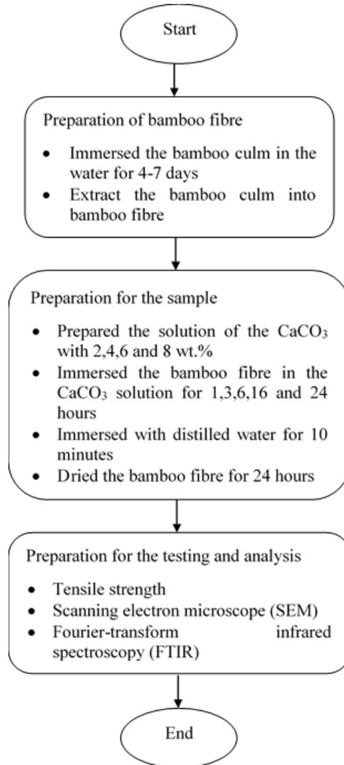
**Figure 1: The flow chart of the methodology for the potential of limestone as preserving agent for a bamboo fibre**
