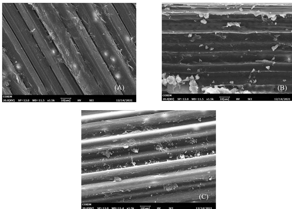
**Figure 5: Morphology of bamboo fibre where (A) untreated/controlled; (B) 4 wt.% concentration of  $\text{CaCO}_3$  for 3 hours; (c) 4 wt.% concentration of  $\text{CaCO}_3$  for 24 hours**
