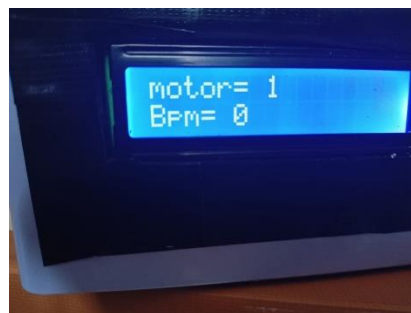
Figure 12: LCD when the virtual switch is HIGH
