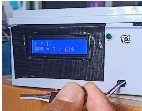
Figure 10: System counting the heart rate
