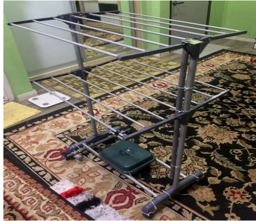
Figure 6: The rain detector for the cloth hanger
