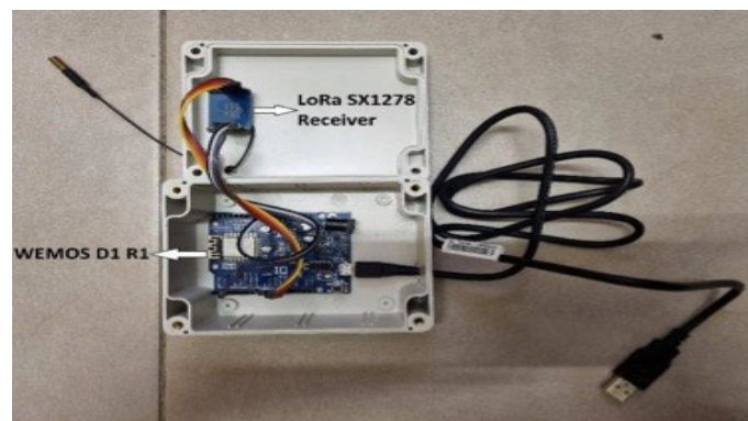
Figure 6: Inside view of Receiver
