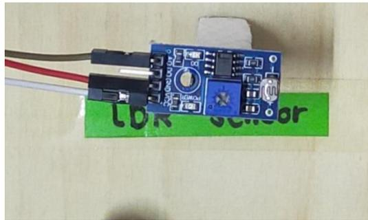
**Figure 4: Element of LDR sensor with a knob sensitivity level**
