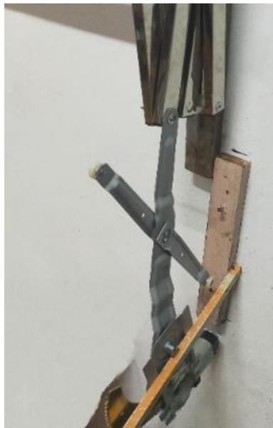
**Figure 8: Integrated Gear and Power Window Motor**
