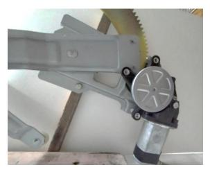
Figure 5: Power window motor and regulator gear
