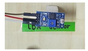
Figure 4: Element of LDR sensor with a knob sensitivity level
