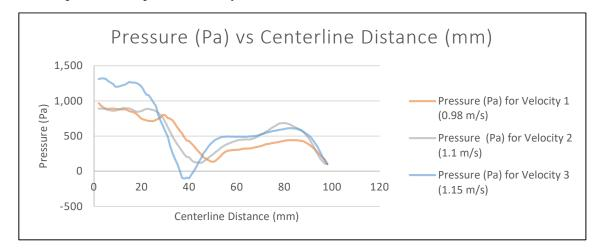
Figure 9: Graph of Comparison of Pressure for Different Inlet Velocity
