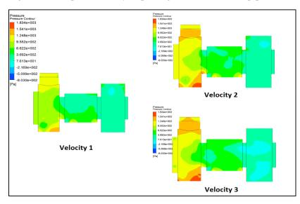
Figure 14: Pressure Contour of Geometry 3 by Using Three Velocity
