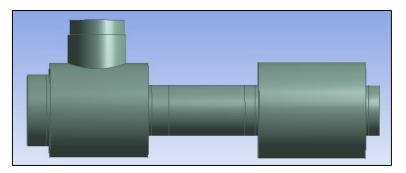
Figure 3: Fluid Domain of Geometry 2 in ANSYS Fluent
