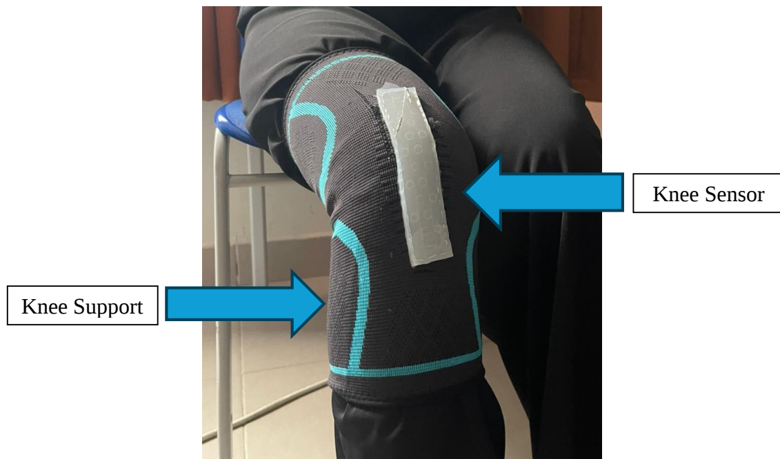
Fig 5 Sensor attached on human knee
