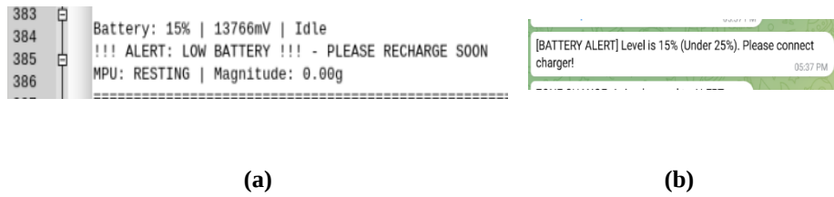
Fig. 9 (a) Battery alert output in the Raspberry Pi terminal (b) Battery alert notification displayed via Telegram
