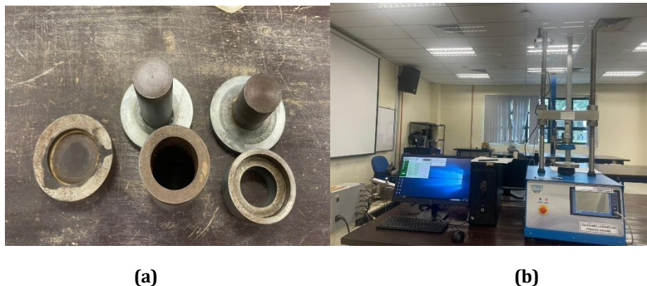
Fig 7 (a) Equipment of Unconfined Compressive Strength (UCS) , (b) UCS Machine test
