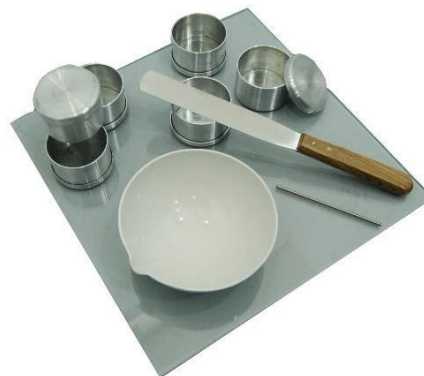
Fig 3 Equipment of Atterberg limit test
