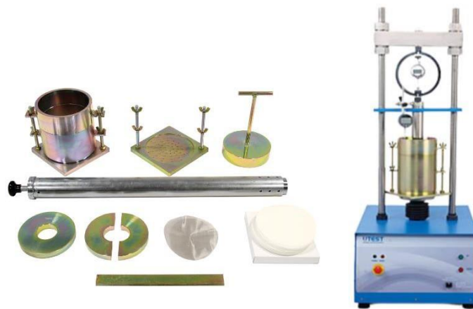
Fig 8 Equipment of California Bearing Ratio (CBR)
