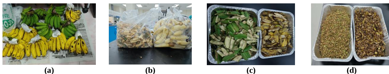
Fig. 1: Preparation of banana peels (a) Collection of yellow and green berangan banana (b) Separated banana pulp and the peels (c) Yellow and green banana peel (d) Chopped yellow and green banana peel in trays.
