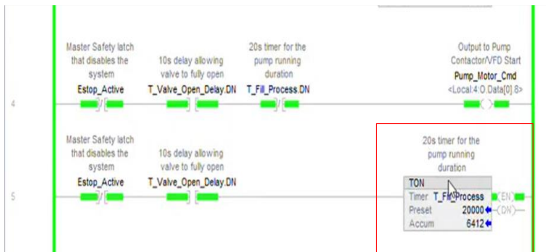
Fig. 2 PLC Timer Instruction showing real-time 20-second filling accumulation
