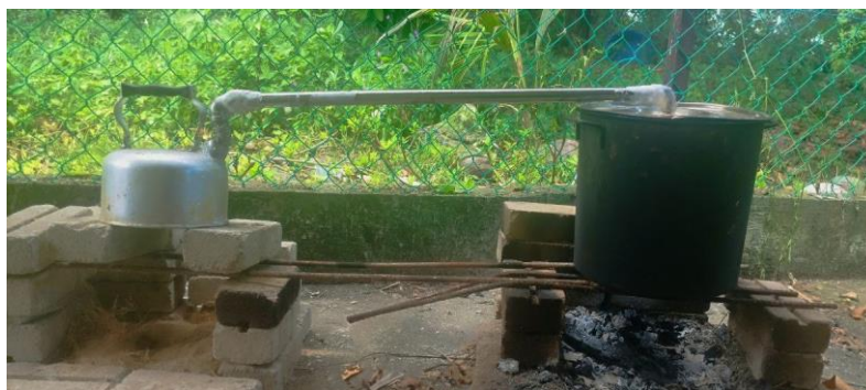
Figure 1: Custom Build furnace for Bamboo Carbonisation
